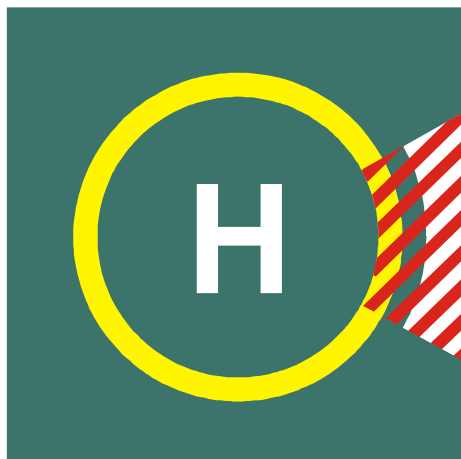
Figure 5-7. Helideck prohibited landing sector marking
